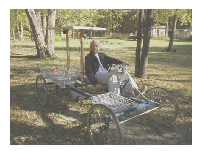
I started designing it in July 03, and finished the basic vehicle to the point of usability in Jan 04. By June 04 I'd installed the solar panel. Over that period I probably spent 30 hours actual "tool time," 30 in front of the computer, and 100 just idly thinking about it. Total cost came to approx \$3900.
